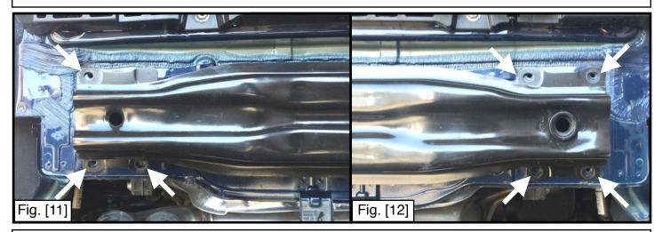
**Step 7.** Thread (1) M8-1.25x40mm Hex Cap Screw through the back of the outside impact bar weld nuts to act as temporary hanging bolts. See Figure [13].
