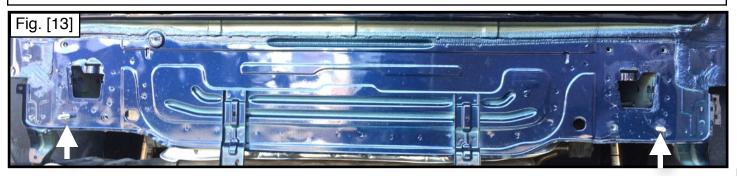
**Step 8.** Place the hitch on to the hanging bolts and then place (1) 1/2"-13x1-1/2" hex cap screw and (1) 1/2" flat washer through the back of the of the inside hole in the vehicle and hitch plate. Secure with (1) 1/2"-13 serrated hex nut and hand tighten. Repeat on opposite side. Ensure that all holes of the hitch frame plates line up with the weld nuts in the vehicle then torque the 1/2" hardware to 75 ft-lbs. See Figure [14]
