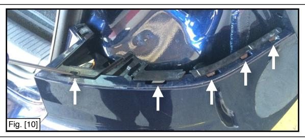
**Step 6.** Discard the foam bar and remove the (7) bolts securing the impact bar in place. Lift the impact bar upward to remove from the vehicle. See Figure [11] & [12].
