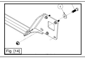
**Step 9.** Place the impact bar over hitch by sliding the driver side lip up into the slot of the EcoHitch. Thread (1) M8-1.25x40mm hex cap screw, (1) 5/16" lock washer, and (1) 5/16" flat washer, into each of the weld nuts on the frame. Remove the temporary hanging bolts and thread into the face of the hitch with (1) 5/16" lock washer and (1) 5/16" flat washer. After all M8 hardware has been hand tightened, torque to 18 ft-lbs. See Figure [15] & [16].
