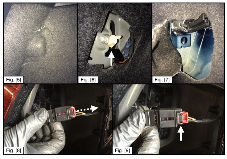
**Step 5.** Starting at the driver side, gently peel the bumper fascia away from the vehicle. Once you reach the tail light section, use a flathead screwdriver or other tool to release the tabs in this section. Move to the passenger side and repeat this process. Unsnap the remaining tabs along the center section of the bumper by pulling rearward. You may need to release the tabs with a flathead in this center section as well. See Figure [10].
